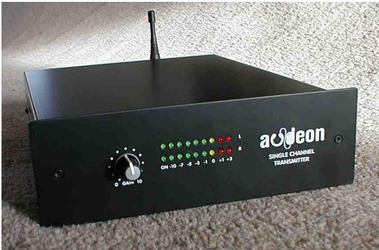
The Single Channel Transmitter is designed as part of the Audeon low power UHF radio system for use in fitness, conference and exhibition centres. It is compatible with the eight channel systems and uses the same transmission frequencies.
